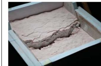
An upcoming part of this project is the analogue modeling of normal fault-joint interaction using brittle, cohesive hemihydrate powder (gypsum).
